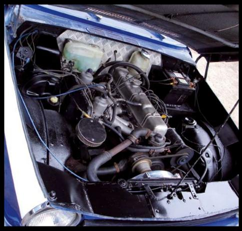
TR6 engine has been squeezed into the Herald's engine bay and mated to the automatic gearbox from a Stag. 🕨
